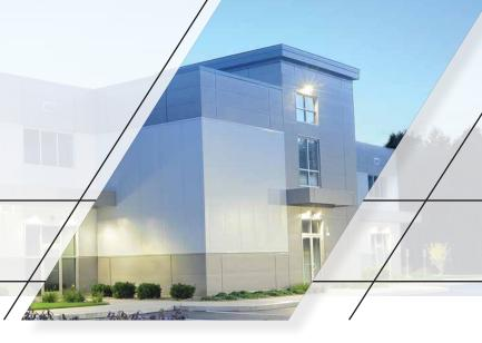
The Metallic CF Santa Fe panel has a flat exterior profile with a heavy, embossed stucco texture that mimics the look of a masonry stucco finish but with the added value of an insulated metal panel. The profile is flush with the warmness of an old-world finish, providing a visually pleasing building.
